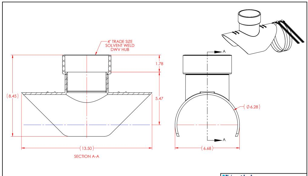
MOLD #: ASM REF. CSA B182.2, B181.2 ASTM D3034 D2665 CAD DATA IS MASTER
